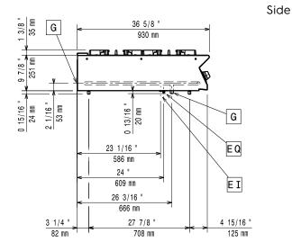
Electrical inlet (power) Gas connection
